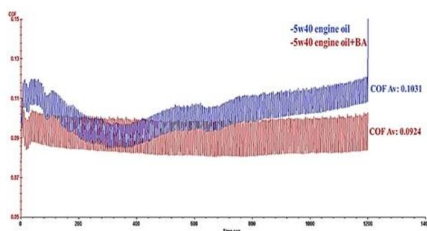
Fig.2 Friction coefficient of 5W-40 engine oil with suspended BA additive via 5W-40 engine oil in ball-on-disk reciprocating tribometer test.
