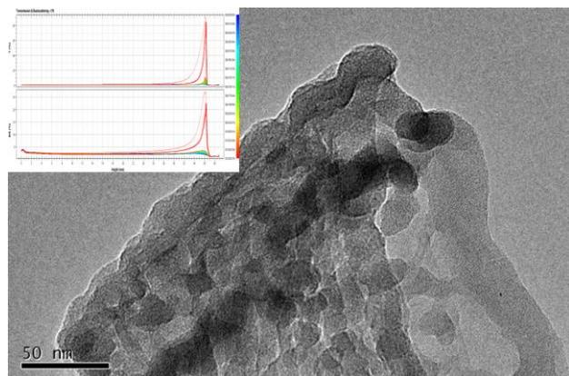
Fig.1 Turbiscan and TEM of BA prepared with Hexane.
