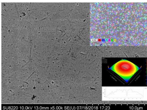
Fig.4 FESEM and 3D roughness of rubbed ball wear track with X-Ray mapping tested with 5W40 engine oil + B.
