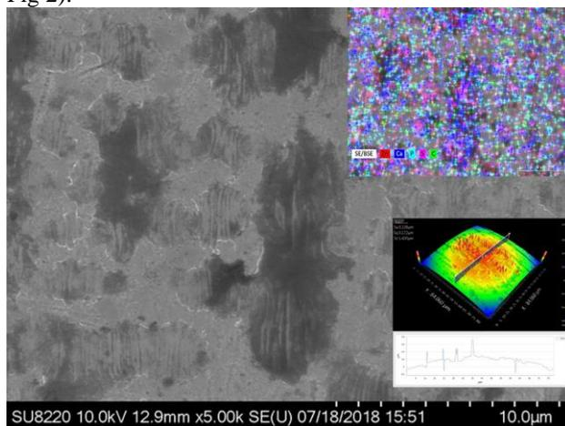
Fig.3 FESEM and 3D roughness of rubbed ball wear track with X-Ray mapping tested with 5W40 engine oil.
